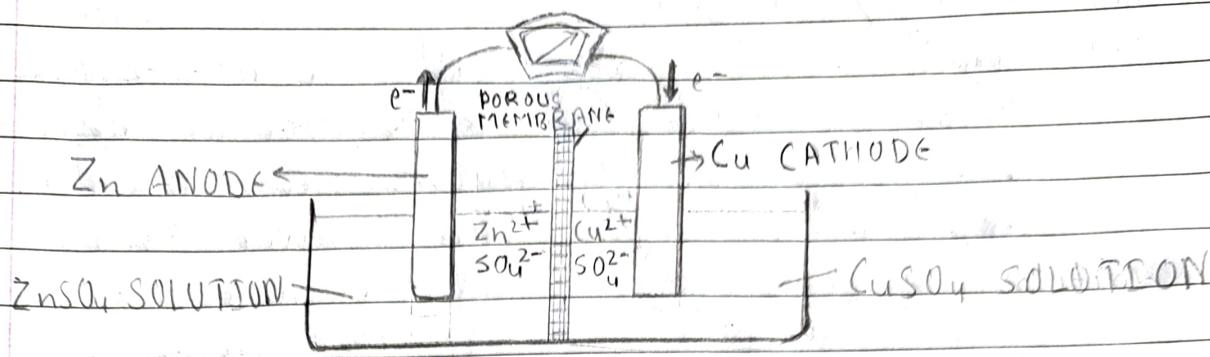
A galvanic cell (with porous membrane)
